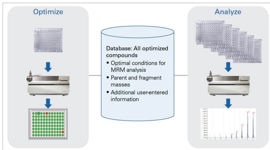
**Figure 1.** The Optimize module in DiscoveryQuant™ Software maximizes compound-dependent parameters and populates a database with these parameters. The Analyze module allows users to create quantitative methods for their analytes based on the stored values in the DiscoveryQuant™ software database. Analyze is also used to create batches, run studies, integrate data, and generate final reports.
