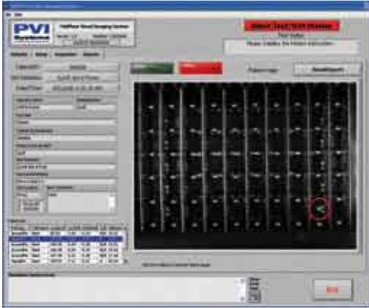
**FIGURE 3.** Images of the pins located on a backplane are presented to the user with failed pins highlighted in red. Once the test is performed, the pass/fail result is indicated to the operator as a green or red status indicator on the PC's user-interface screen. Regardless of whether the backplane fails or passes the test, a report is generated in a test folder and images are saved as raw .bmp files.
