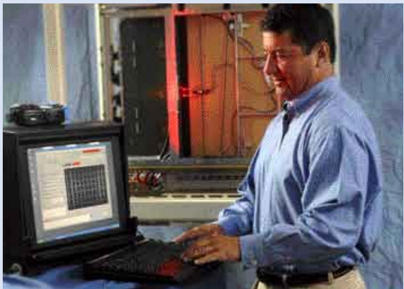
To inspect the backplane connectors on a mainframe storage server, PVI Systems has developed a smart imaging board that uses a motor-driven embedded CCD camera controlled with a PC-based motion-control and imaging subsystem.
